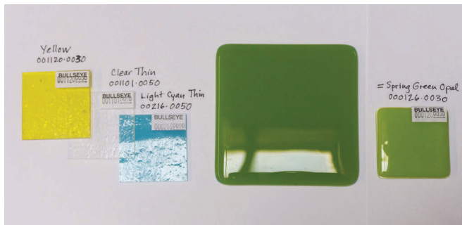
TOP: Yellow 001120-0030; MIDDLE: Clear Thin 001101-0050; BASE: Light Cyan Opal Thin 000216-0050. Requires Clear Thin between colors to prevent a dark color reaction.
